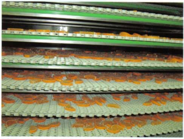
Schüttgut-Pufferung/buffering of bulk products
